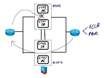
The ASA1 appliance doesn't have any state data for the particular packet in our example. The packet will be dropped.
