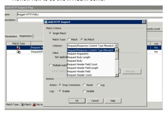
The "Multiple matches" section has predefined traffic classes to detect covert channeling / tunnels ...
