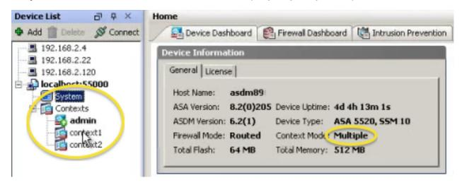
Notice the System section highlighted above – it uses the admin context to derive it's settings – these are both present by default. Even though the admin context is "special", it can still be configured and assigned just like any other context.
