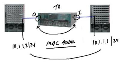
Traffic forwarding is no longer based on IP addresses as it is in Routed Mode. Our traffic forwarding is based on **Layer 2 (MAC addresses)**. This is referred to as **Secured Transparent Bridging** between the two interfaces.
